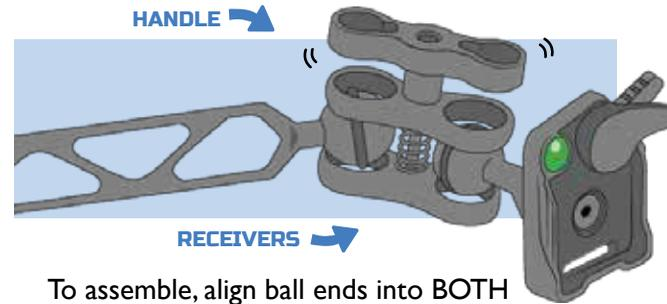
To assemble, align ball ends into BOTH Joint-Clamp receivers and tighten the handle. Be careful not to overtighten Joint-Clamps during the initial assembly.
